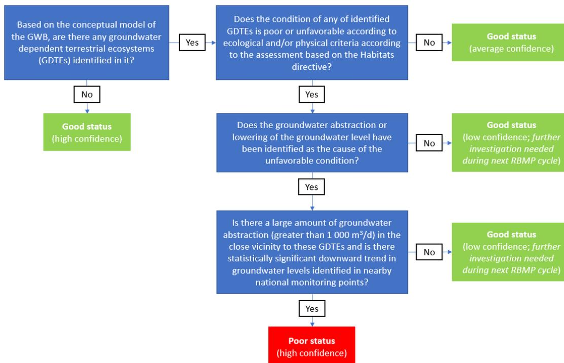
FIGURE 1.8.2.1.4 Flow diagram of the GDTEs assessment test (modified after Marandi et al., 2020)
