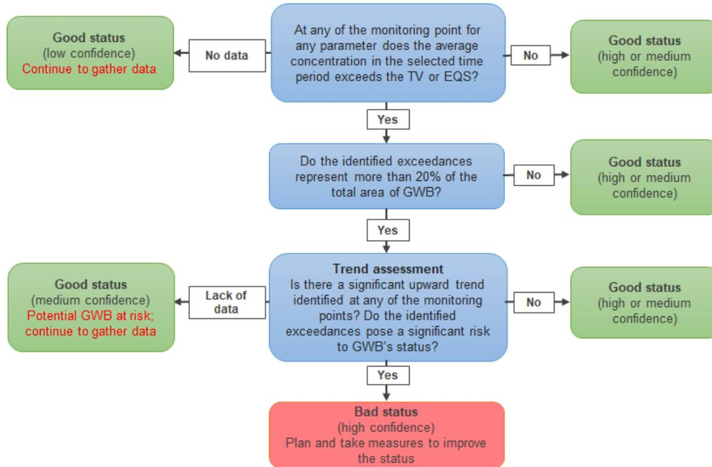
FIGURE 1.8.1.2.2 Schematic procedure for tests used to assess the chemical status of GWB (modified after LVGMC, 2021)
