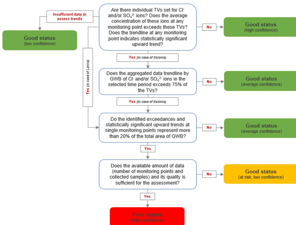
FIGURE 3.5.1.2.1 Flow chart diagram of the harmonized Estonian-Latvian approach of the saline or other intrusions assessment test (Test 2)
