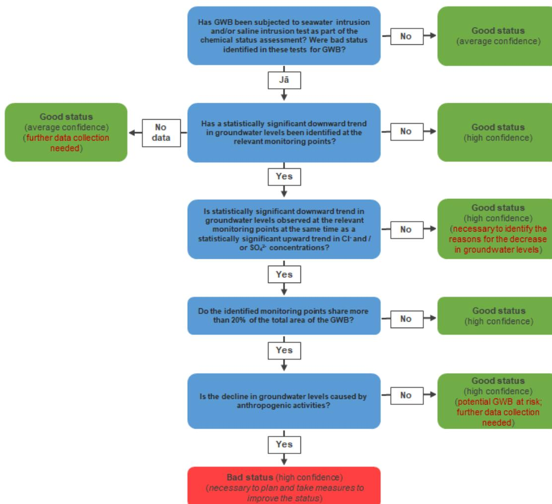
**FIGURE 1.8.2.2.2 Schematic procedure of saline or other intrusion tests**
