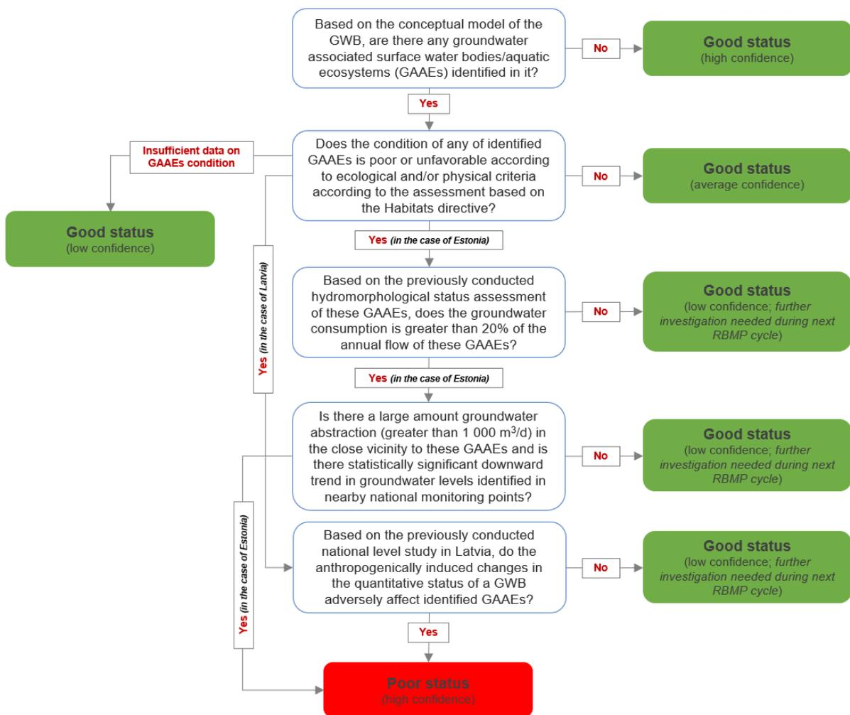
FIGURE 3.5.2.3.1 Flow chart diagram of the harmonized Estonian-Latvian approach of the associated SWBs assessment test (Test 8)
