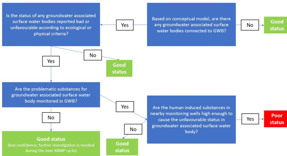
**FIGURE 1.8.1.1.4 Flow diagram of the surface waters test**
