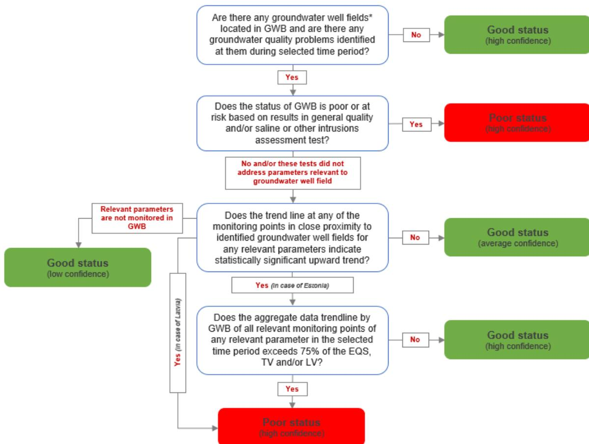
FIGURE 3.5.1.5.1 Flow chart diagram of the harmonized Estonian-Latvian approach of the DWPA's assessment test (Test 5)
