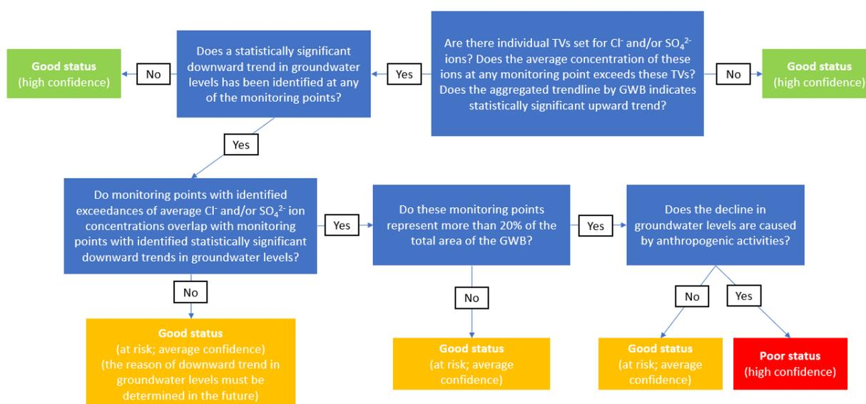
FIGURE 1.8.2.1.2 Flow diagram of the saline or other intrusions assessment test
