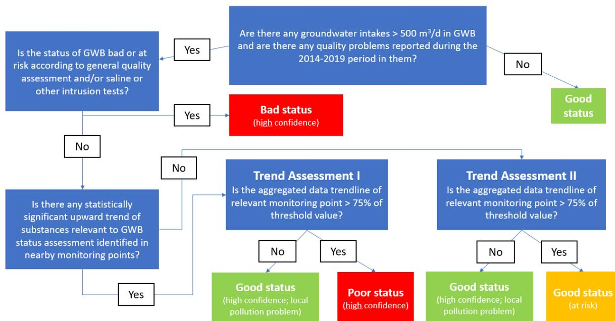
**FIGURE 1.8.1.1.6 Flow diagram of the DWPA test**
