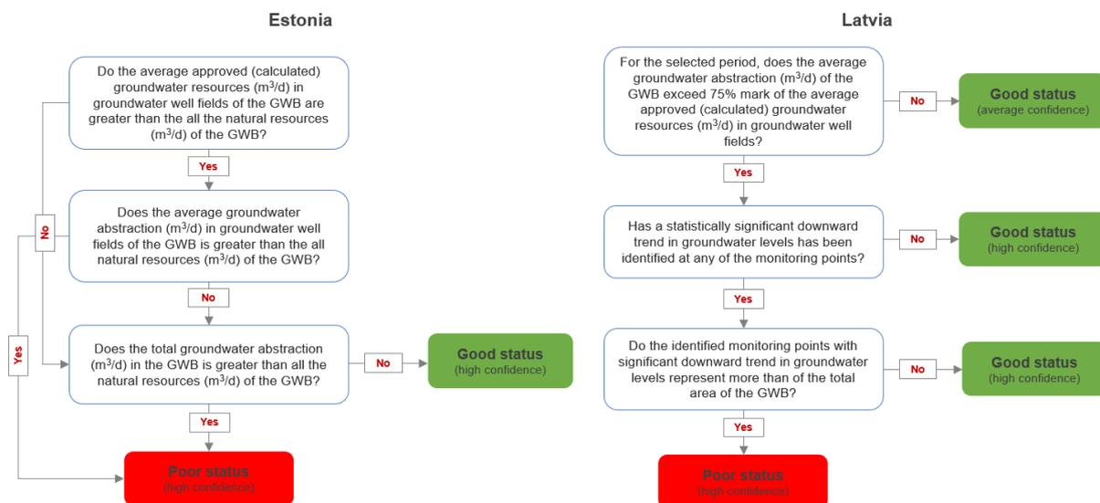
FIGURE 3.5.2.1.1 Flow chart diagrams of the Estonian and Latvian approaches of the water balance assessment test (Test 6)
