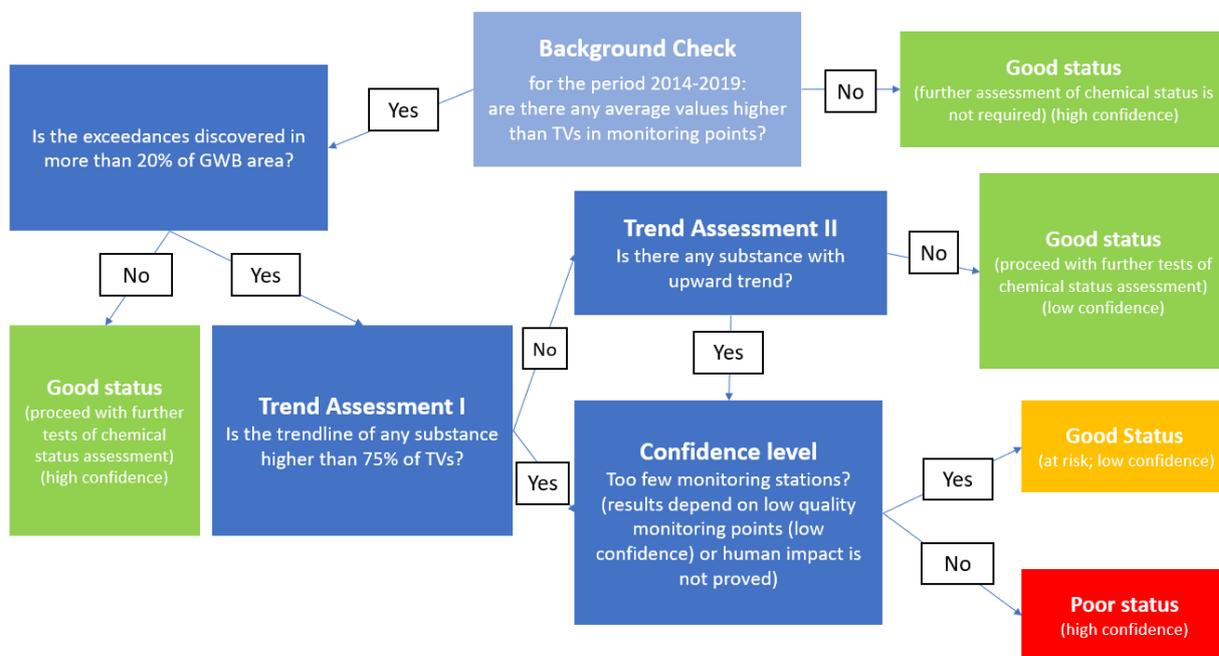
FIGURE 1.8.1.1.1 Flow diagram of the background check and the general quality assessment test
