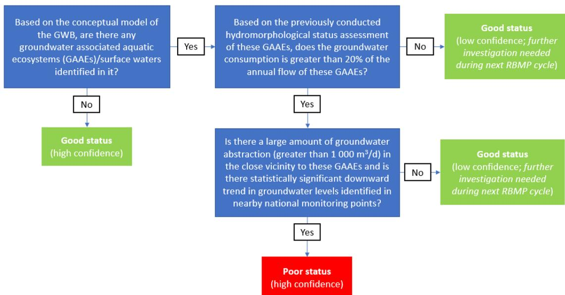
FIGURE 1.8.2.1.3 Flow diagram of the surface waters assessment test
