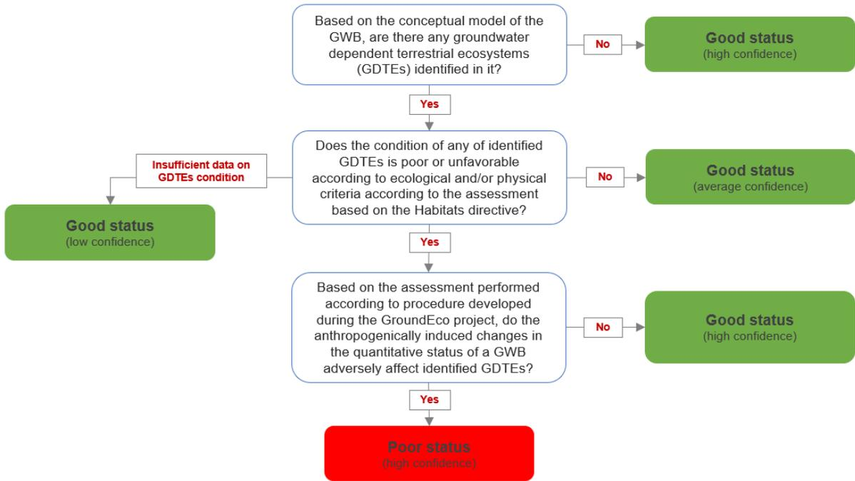
FIGURE 3.5.2.4.1 Flow chart diagram of the harmonized Estonian-Latvian approach of the GDTEs assessment test (Test 9)
