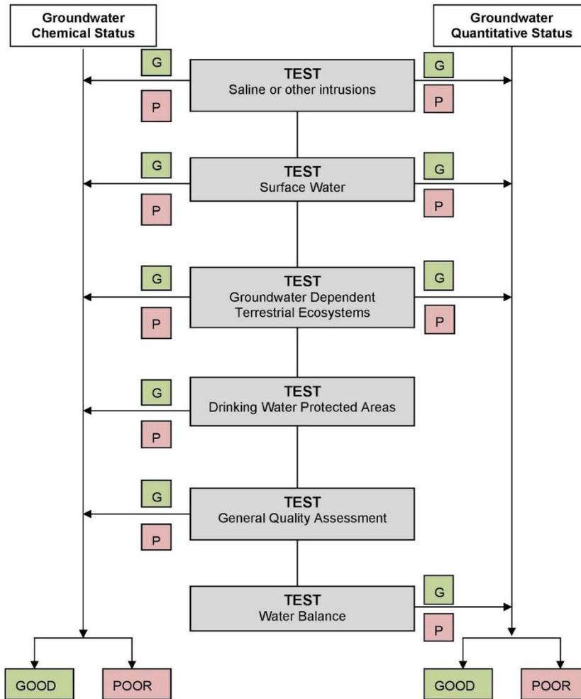
FIGURE 1.8.1 Overall procedure of tests for assessing groundwater status (EC, 2009)
