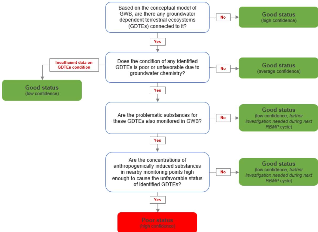
FIGURE 3.5.1.4.1 Flow chart diagram of the harmonized Estonian-Latvian approach of the GDTEs assessment test (Test 4)
