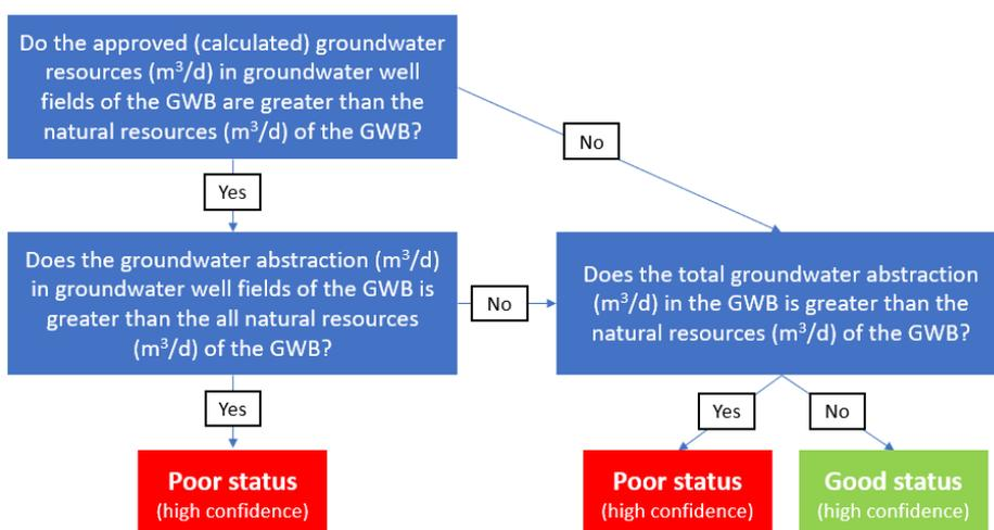
**FIGURE 1.8.2.1.1 The flow diagram of the water balance test**
