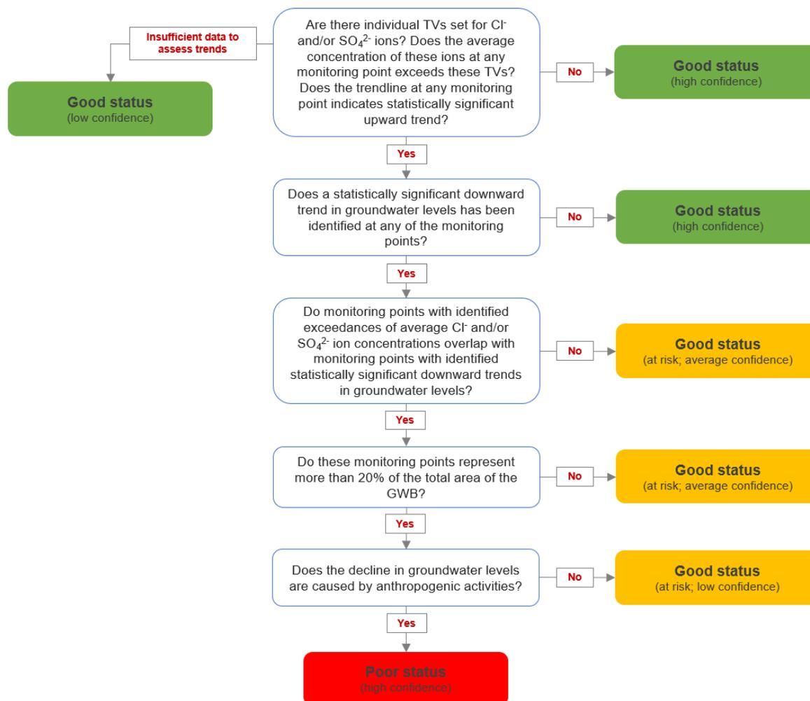
FIGURE 3.5.2.2.1 Flow chart diagram of the harmonized Estonian-Latvian approach of the saline or other intrusions assessment test (Test 7)
