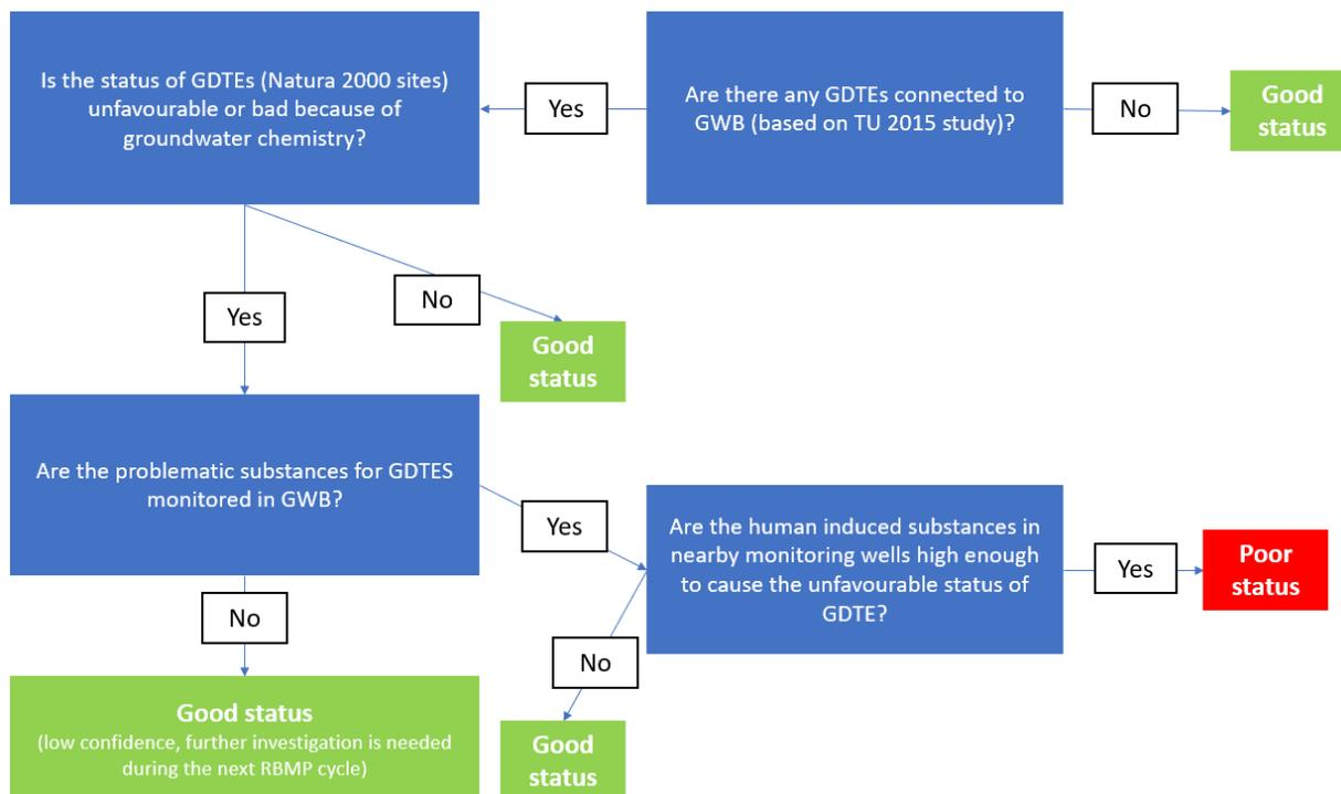
FIGURE 1.8.1.1.5 Flow diagram of the GDTEs test (modified after Marandi et al., 2020)
