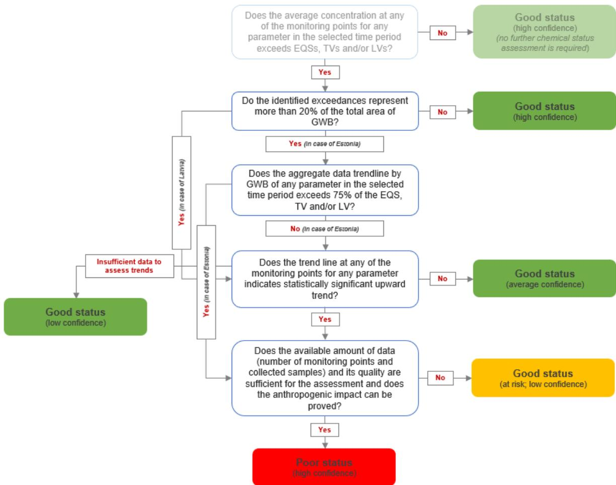
**FIGURE 3.5.1.1.1 Flow chart diagram of the harmonized Estonian-Latvian approach of the general quality assessment test (Test 1)**
