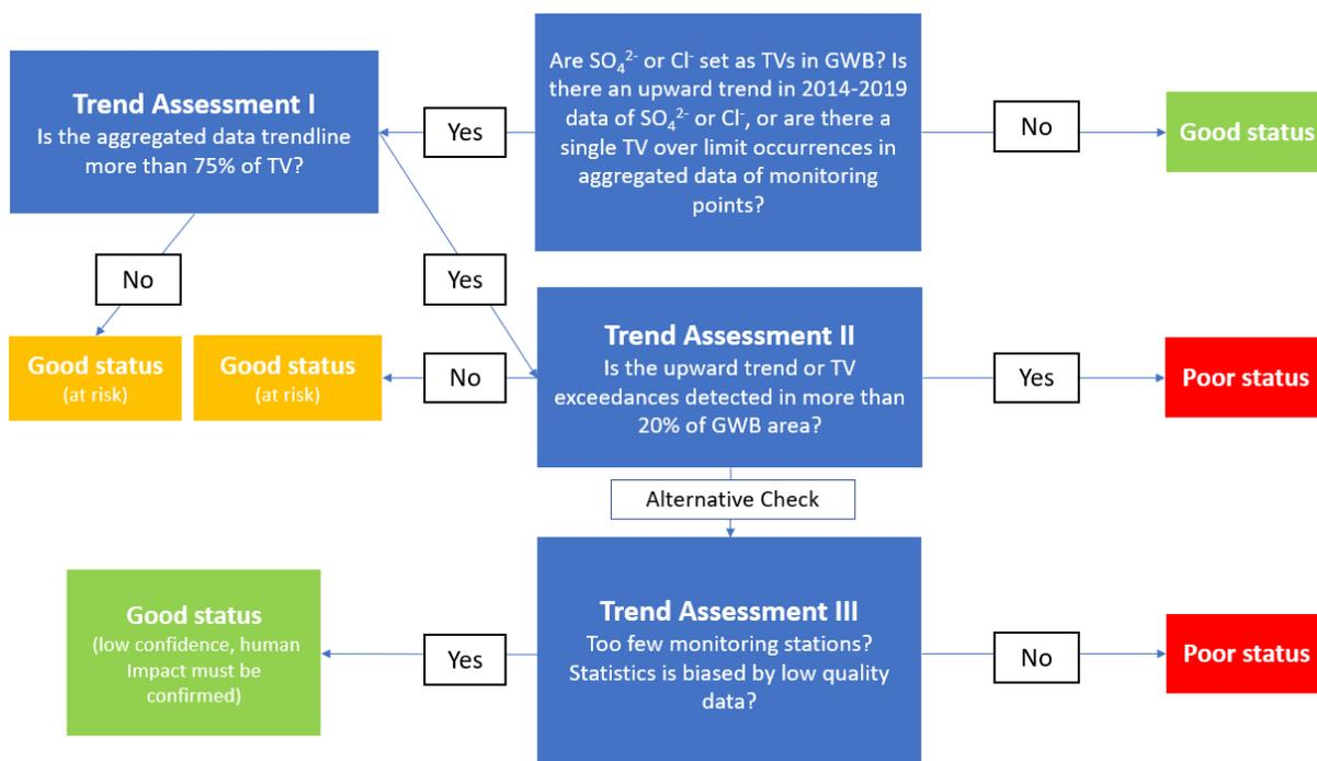
**FIGURE 1.8.1.1.3 Flow diagram of the saline or other intrusions test**
