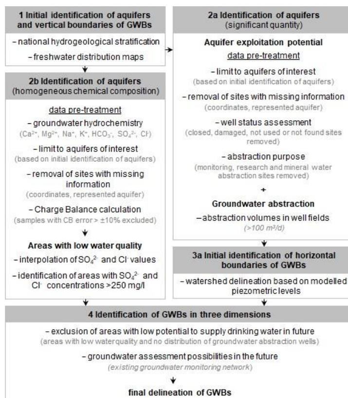
FIGURE 1.1.2.1 Schematic flowchart illustrating main steps and data pre-treatment procedures for GWB delineation in Latvia (Retiķe, 2017)
