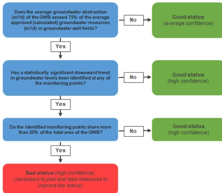
**FIGURE 1.8.2.2.1 Schematic procedure of groundwater balance test**
