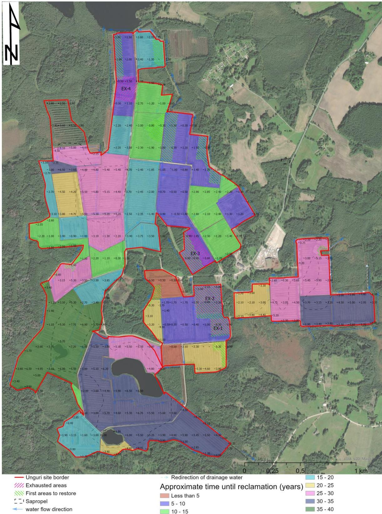
Figure 8. Unguri peat production site approximate time until after-use and peat depth according to the geological survey points
