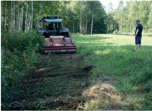
Fig. 21.4.5. Shrub root grinding in Krustkalni Nature Reserve. The principle of shredder operation is similar to the shredder provided in Fig. 21.4.4, but it is slightly wider. This type of shredder is more suitable for mineral soils. Photo: A. Namatēva.
