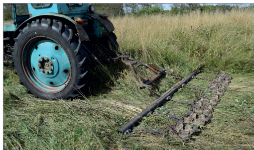
Fig. 21.3.9. A toothless drag-harrow, which enables smoothing of molehills and wild boar rootings, as well as sedge tussocks, if the harrowing is performed in the autumn in conditions of frost, when the tussocks are fragile. Photo: S. Rüşîa.
