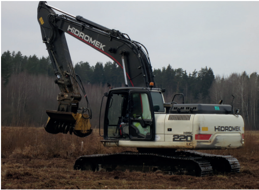
Fig. 21.4.4. Grinding of shrub roots in peat soils in the Dviete floodplain meadows in winter, when the ground is frozen. A tracked tractor is used to enable movement on soft ground. Photo: S. Rūsiņa.
