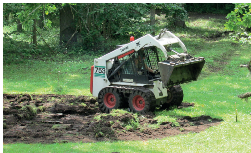
Fig. 21.7.2. Removal of turf with an excavator. Photo: A. Priede.
